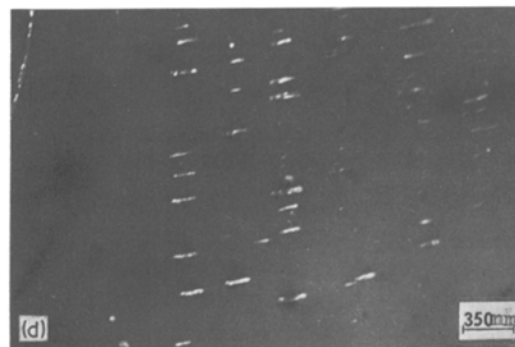
Figure 4 Microstructure of Sn-10 at.% Sb alloy annealed 10 min at 373 K: (a) TEM bright-field micrograph; (b) diagram of the electron diffraction pattern; (c) and (d) dark-field micrographs by diffracted beams from matrix and precipitates and by beams from precipitates only, respectively.
